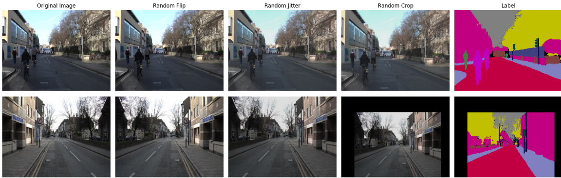
Figure 4.2 Example of two images going through the augmentation process step by step, the images are randomly flipped, jittered, and cropped. Note that the label and the image go through the same augmentation but with random parameters each time. Image augmentation is computed in parallel to the main training loop
